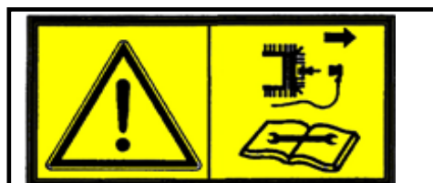
Before doing maintenance remove the spark plug.
